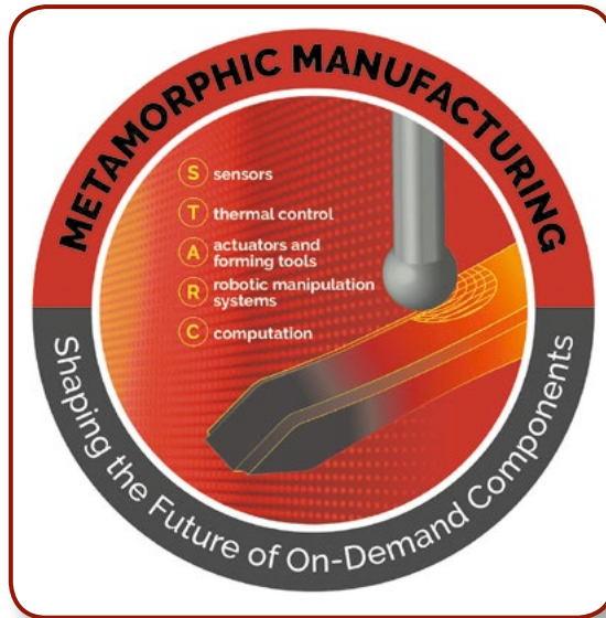
Figure 1. A visual synopsis of the five fundamental elements of metamorphic manufacturing. ( Metamorphic Manufacturing: Shaping the Future of On-Demand Components , 2019, p. xxiv.)
