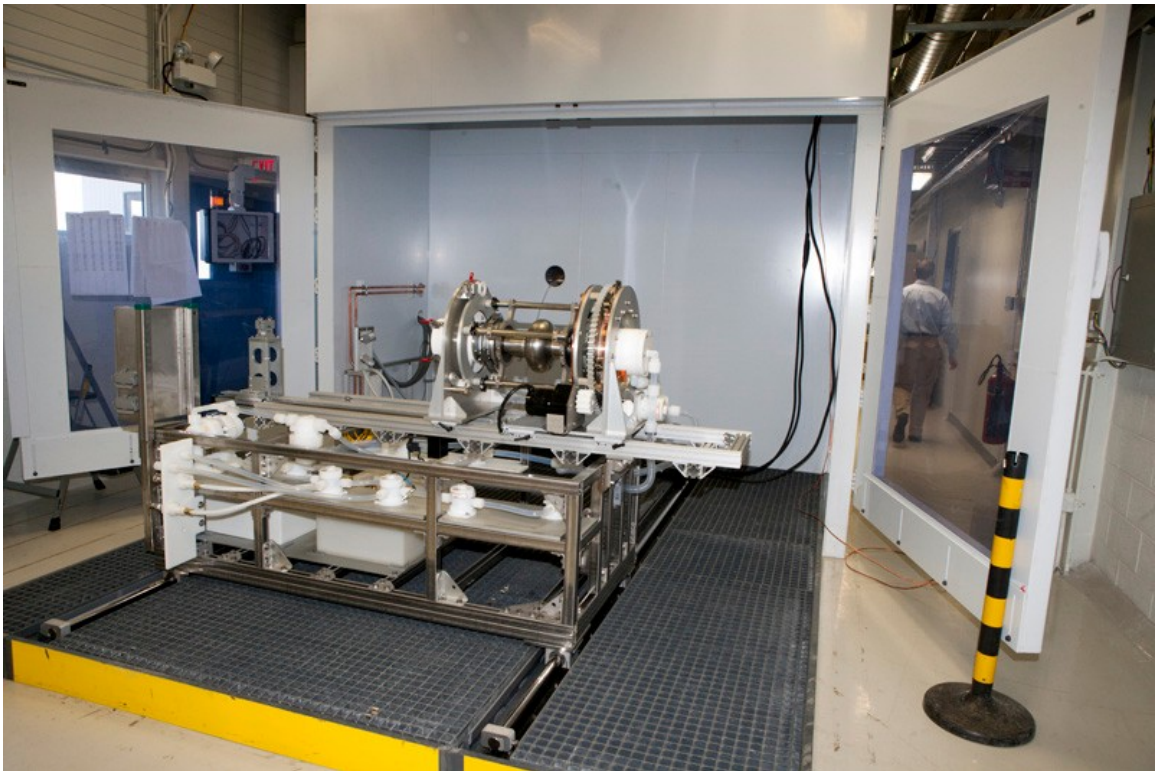
Fig. 2.2: Electropolishing set up at Fermilab showing an assembled niobium single cell cavity [9].
