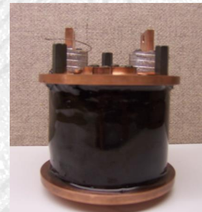
Small Scale Model Undulator for International Linear Collider
