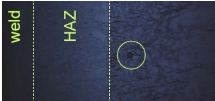
Figure 1.7 Defects near the welded region and the heat-affect zone (HAZ) of the cavity surface [28]
