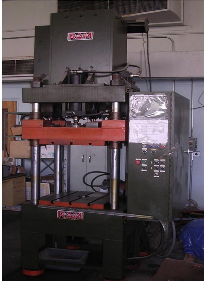
Figure 3.2 The OSU's hydraulic press for bulge test
