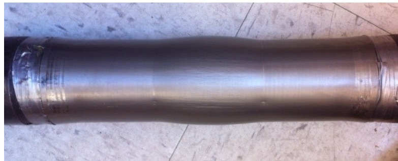
Figure 3.14 Bulge formed in the reactor grade Nb tube heat treated for 2h/1000°C
