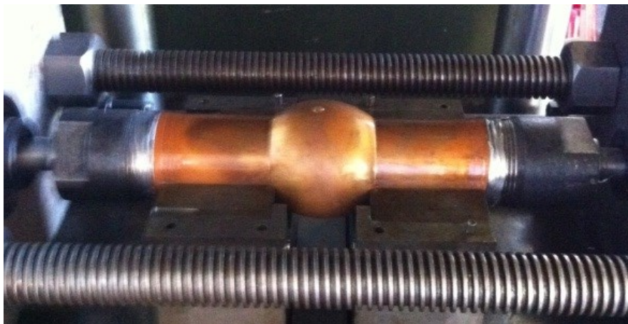
Figure 3.11 Bulge formed in the OFHC Cu tube heat treated for 2h/500°C
