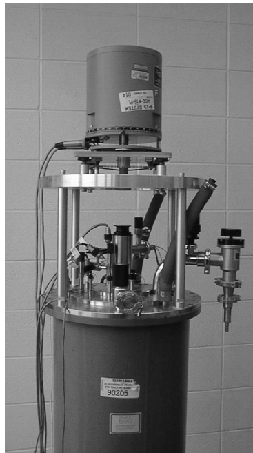
Fig. 3.4. 9 T VSM, head, mounting, and dewar.
